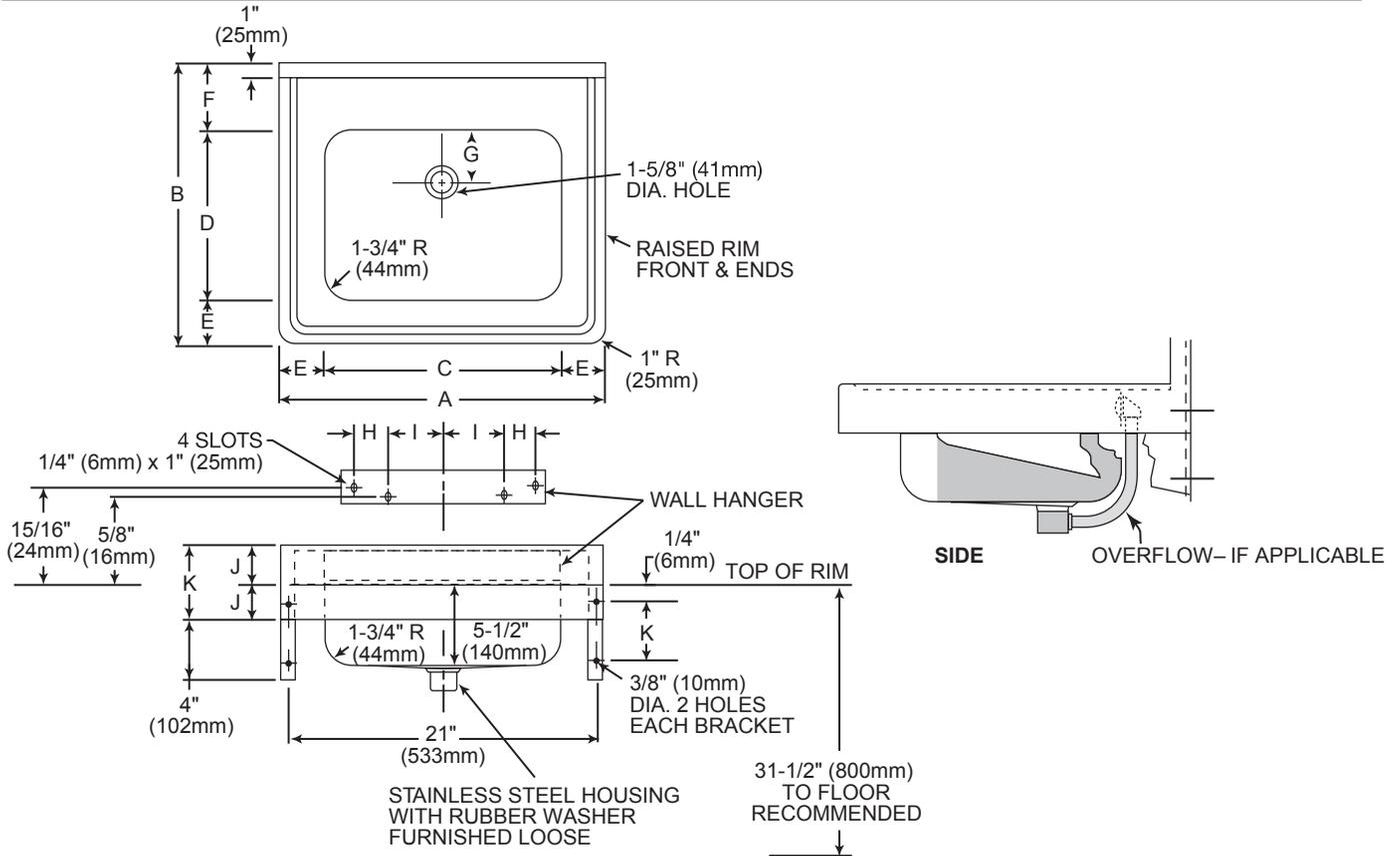
**HOLE DRILLING CONFIGURATIONS**
