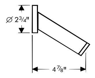
Female pipe fitting recessed 3/8" behind surface finished wall
