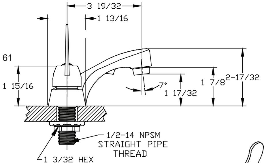
The lavatory centerset is designed with a solid cast brass body with shanks located on 4-inch centers for supply connections and mounting. The stems are all brass with a double O-Ring seal and rubber seat washer. The 6-inch elbow blade handles are brass with a color coded hot and cold index. The faucet body is polished and copper, nickel and chrome plated. The faucet is fitted with a water saving aerator that limits the flow rate.
