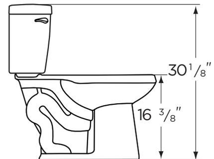
THIS FIXTURE QUALIFIES ACCORDING TO ASME TEST PROCEDURES AS A HIGH EFFICIENCY WATER CLOSET WITH AN AVERAGE CONSUMPTION OF 1.28 gpf (4.8 Lpf) OR LESS.
