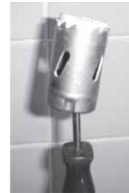
5. After the initial 1-1/4" (30mm) hole is made through the tile, stop, and eject the tile from the drill bit.
