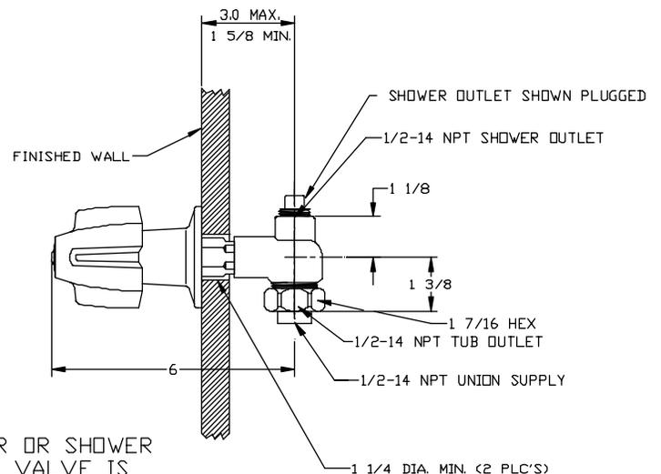
NOTE: THE BATH VALVE MAY BE USED FOR A TUB FILLER OR SHOWER VALVE. DO NOT USE AS BOTH UNLESS THE BATH VALVE IS CONNECTED TO A DIVERTER SPOUT WITH A TWIN ELL.
