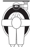
2. As the user enters the beam's effective range (22" to 42") the beam is reflected into the OPTIMA Plus Scanner Window and transformed into a low voltage electrical circuit. Once activated, the Output Circuit continues in a "hold" mode for as long as the user remains within the effective range of the Sensor.
