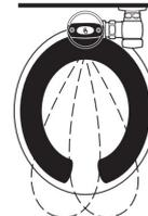
3. When the user steps away from the OPTIMA Plus® Sensor, the circuit waits 3 seconds (to prevent false flushing) then initiates an electrical signal that operates the Solenoid. This initiates the flushing cycle to flush the fixture. The Circuit then automatically resets and is ready for the next user.
