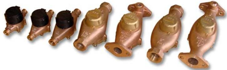
**INTRODUCTION:** ZENNER PERFORMANCE Multi-jet Water Meters utilize a magnetically driven multi-jet design. They are designed to measure cold potable water where flow is in one direction only in residential, commercial, and industrial settings.
