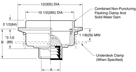
Fig. 3970C . . . CAULK OUTLET Fig. 3970Y ... NO-HUB OUTLET
