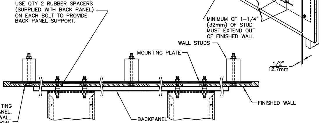
\*FINISH WALL OVER MOUNTING PLATE AND BEHIND BACKPANEL, MAKE SURE THAT FINISHED WALL EXTENDS WITHIN THE BRACKET/BOWL MOUNTING HOLES (TO PROVIDE SURFACE AREA FOR RUBBER SPACERS TO CONTACT).
