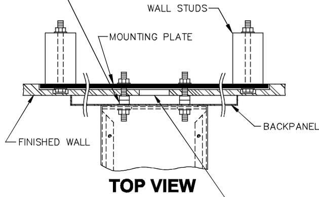
\*FINISH WALL OVER MOUNTING PLATE AND BEHIND BACKPANEL. MAKE SURE THAT FINISHED WALL EXTENDS WITHIN THE BRACKET/BOWL MOUNTING HOLES (TO PROVIDE SURFACE AREA FOR RUBBER SPACERS TO CONTACT).
