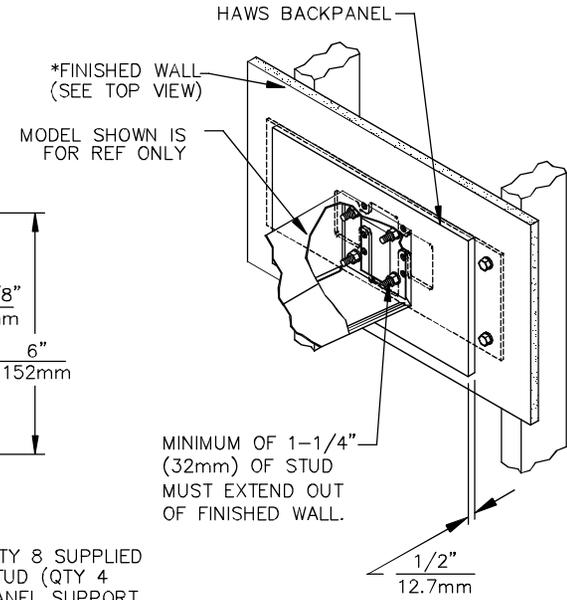
USE QTY 2 RUBBER SPACERS(QTY 8 SUPPLIED WITH BACK PANEL) ON EACH STUD (QTY 4 SUPPLIED) TO PROVIDE BACK PANEL SUPPORT.
